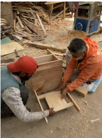
The modern looking but traditional dry toilet consists of a box for the soil and a seat. The first sets were installed at Hemis Monastery.
