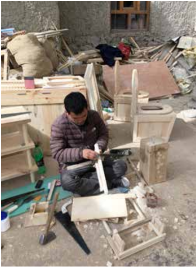
The modern looking but traditional dry toilet consists of a box for the soil and a seat. The first sets were installed at Hemis Monastery.
